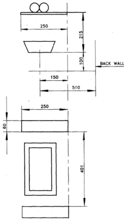
FIG. 3 METHOD OF SUPPORT OF TEST PIECE
